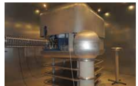
Figure 1: The 500kV single ended accelerator. RUBION operates ion facilities from 5kV table top system to a 4 MV tandem accelerator with up to 60 m beam lines.
